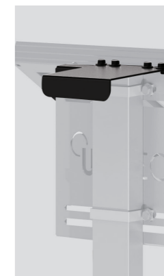
Easy installation system Its upper cap relieves the weight of the installation so that their mounting can easily be done alone, without extra assistance. This cap can be removed afterwards for a fixation on the middle of the pole with a maximum of 130mm diameter. For UNIFIX 100S /150S /200S.
