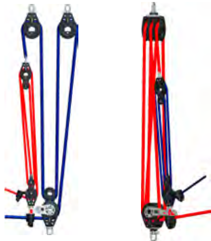
Examples of main sheet tackles with fine tuning.
