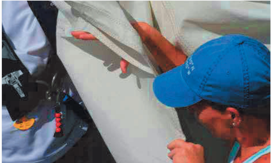
Stitching is usually the first to fail on old sails as ultra-violet (UV) rays take their toll.
