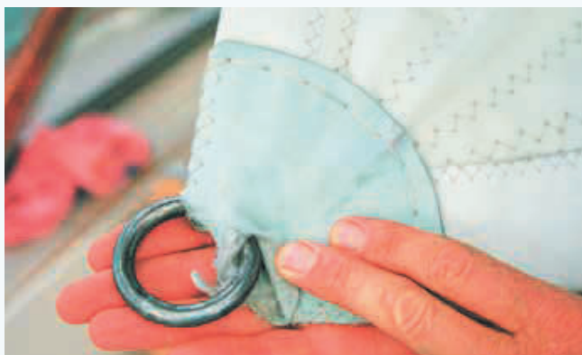
Staggering the stitches on a clew repair avoids creating a perforated line that can create a rip-on-the-dotted line effect under load.
