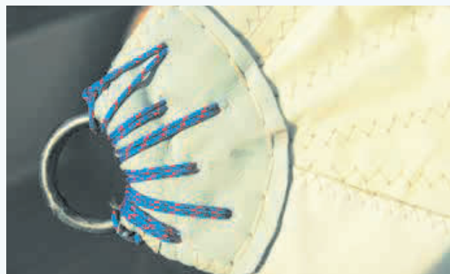
Staggering the stitches on a clew repair avoids creating a perforated line that can create a rip-on-the-dotted line effect under load.
