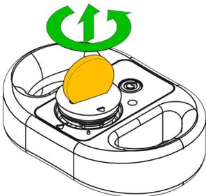
Replace the CR2032 battery with equivalent. Do not use non-standard batteries or other sizes, as this can cause damage.
