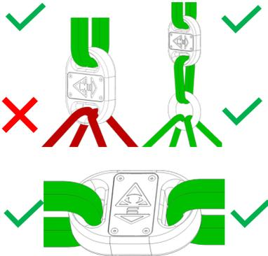
Figure 1 Incorrect and correct strop loading
